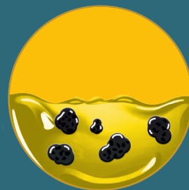
Contaminants that have been attracted by Alu Treater and flocculated into larger filterable clusters
